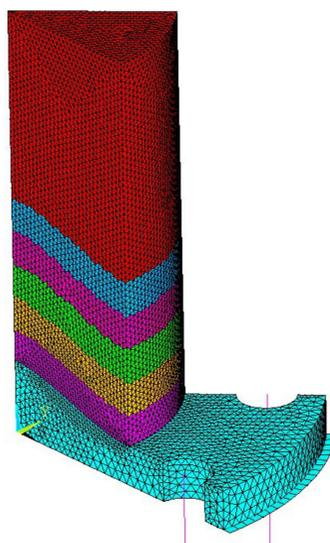
The effective elastic properties of the lattice material were associated to an equivalent homogeneous solid that replaces the lattice domain. These orthotropic properties were obtained from the structural analysis of a single representative volume element: the unit cell.
